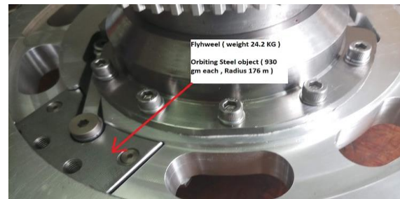
Figure 2b : Counter weights of 930 grams as inside flywheel
