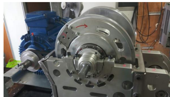
Figure 2c : Flywheel 24.2 kg with 2 counter weight .92 kg
